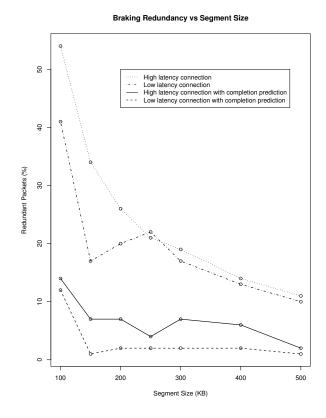
Figure 2: Braking redundancy of a network coding client. The top two lines use the naive braking method and thus experience a high level of redundancy. The lower lines use predictive braking to estimate completion times, resulting in lower levels of redundancy. The low latency tests were performed on a local network (avg. latency: 0.2ms) and the high latency tests over the Internet (avg. latency: 52ms)
