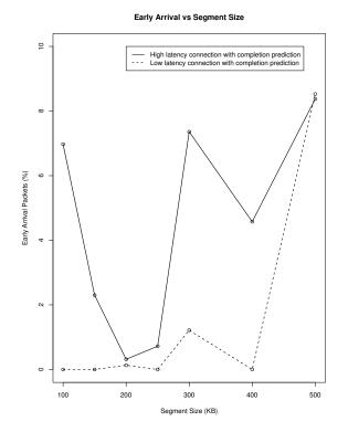
Figure 3: Packets arriving while a previous segment is still incomplete. Ideally the percent of early arrivals will remain low when using completion prediction, so that segments finish quickly and the streaming rate is not affected. The low latency tests were performed on a local network (average latency: 0.2ms) and the high latency tests over the Internet (average latency: 52ms)
