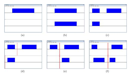
Figure 5: A sequence of pulse insertions and synchronizations: (a)  $90^{\circ}$  hard pulse is added to the first channel. (b)  $90^{\circ}$  hard pulse is added to the second channel. (c)  $180^{\circ}$  hard pulse is added to the first channel. (d) markers are added to both channels. (e) both markers are synchronized. (f)  $180^{\circ}$  hard pulse is added to the second channel.
